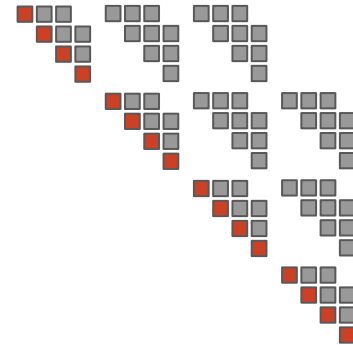
Depiction of naive parallelization: all terms for the red cells are evaluated in parallel
