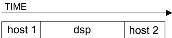
**Figure 3.** Block diagram of a single iteration of the inner loop of Co-Bind, running on the host-DSP platform.
