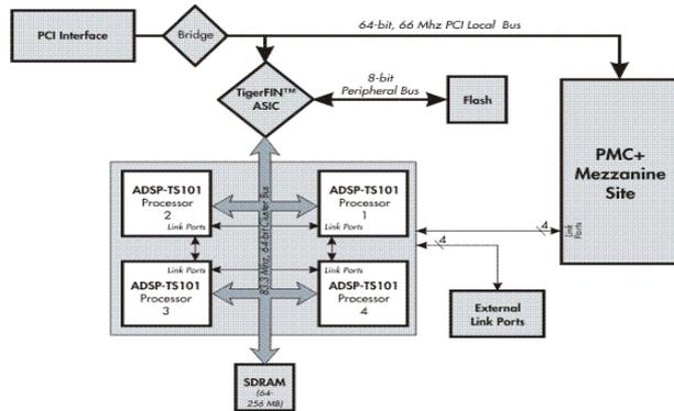
**Figure 1.** Architecture of the BittWare Tiger-PCI board, picture taken on the web site www.bittware.com.
