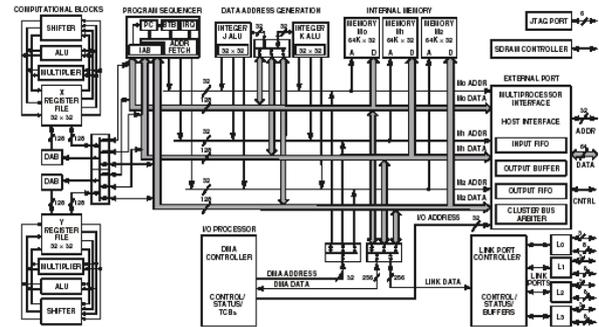
**Figure 2.** Functional block diagram of the TigerSHARC ADSP-TS101S DSP processor.
